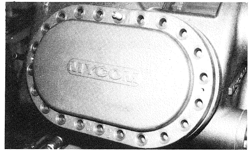
Fig. 79 Mounting air-cooled head cover WB
