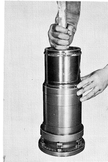
Fig. 69 Inserting piston into sleeve
