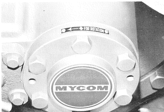
Fig. 10 Compressor rotation direction plate
