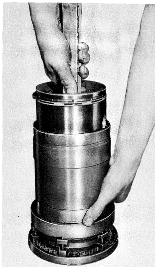
Fig. 44 Removing piston from cylinder sleeve
